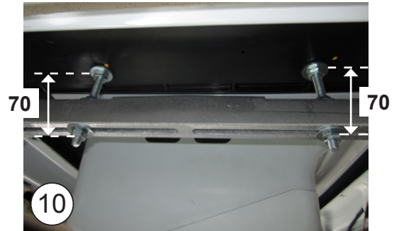
Left side view in vehicles with Space, Mega Space and Giga Space cabs
