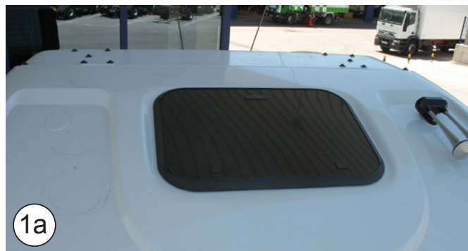
Stralis Cabin before 2008: 40 x 40 EPDM joint
