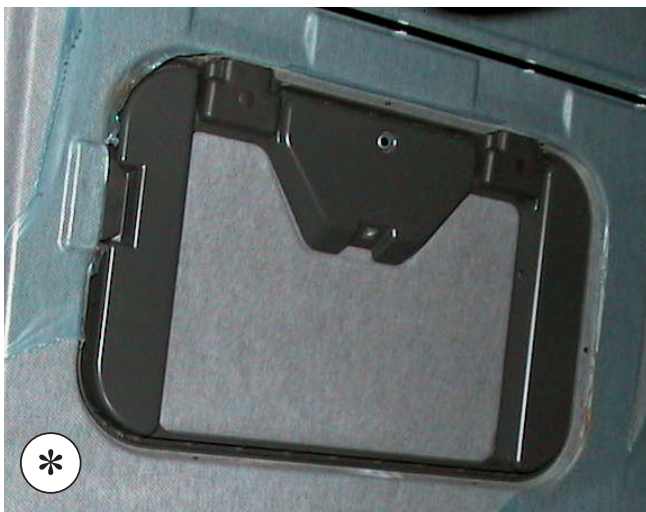
Standard Cabin and Stralis Cabin since 2008: 30 x 25 EPDM joint
